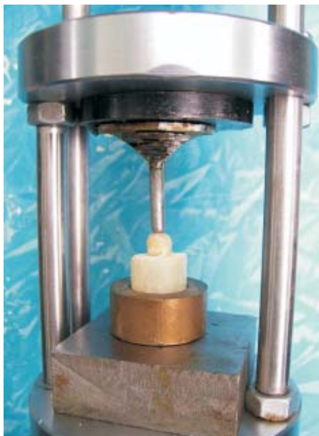
FIGURE 2 - Specimen under compressive load
