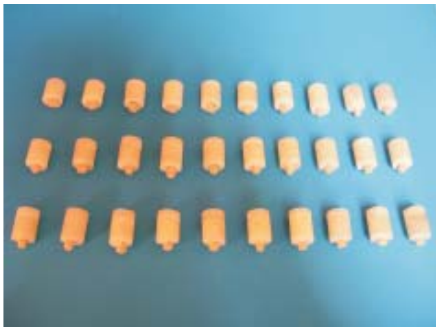
FIGURE 1 - The roots are embedded, 2 mm beneath CEJ in auto polymerized acrylic blocks, while an even 0.2 mm thickness of Impergum functions instead of natural PDL around the specimens
