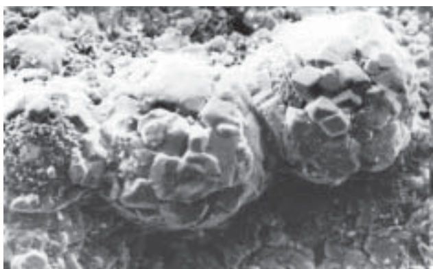
FIGURE 4 - SEM Photographs (x 3500) of the high-copper dental amalgam GS.80
