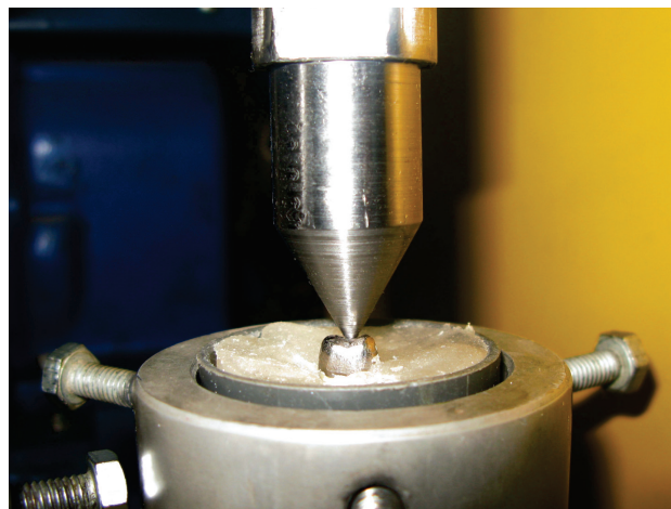
Figure 2 - Schematic illustration of Fatigue loading test Source: Research data.
