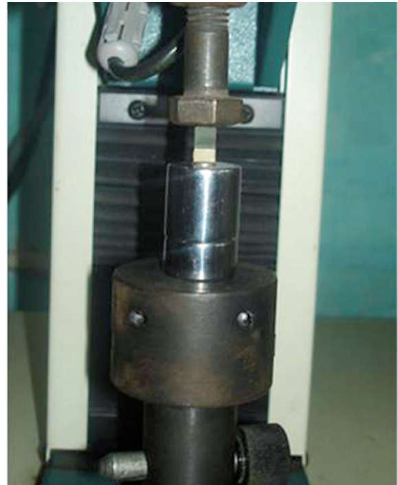
Figure 3 - Specimen mounted in jig for shear testing in universal testing machine
