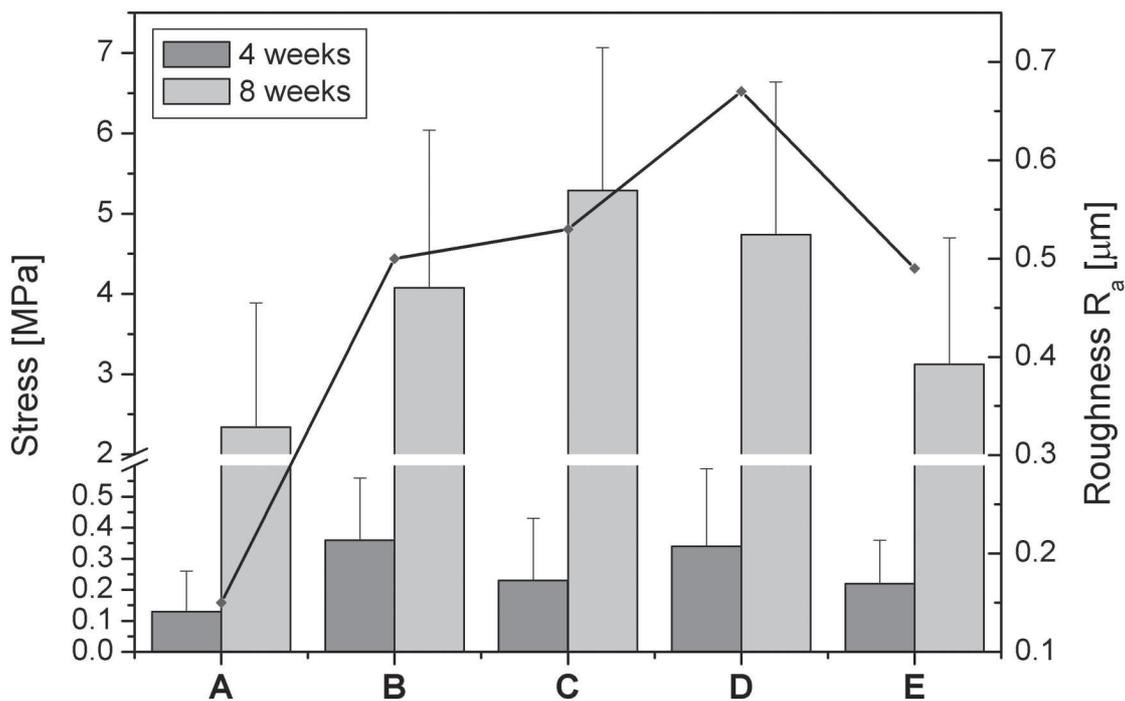
FIGURE 5 - Comparison between the ultimate stress mean values and the roughness ( $R_a$ ) mean values for both healing times
