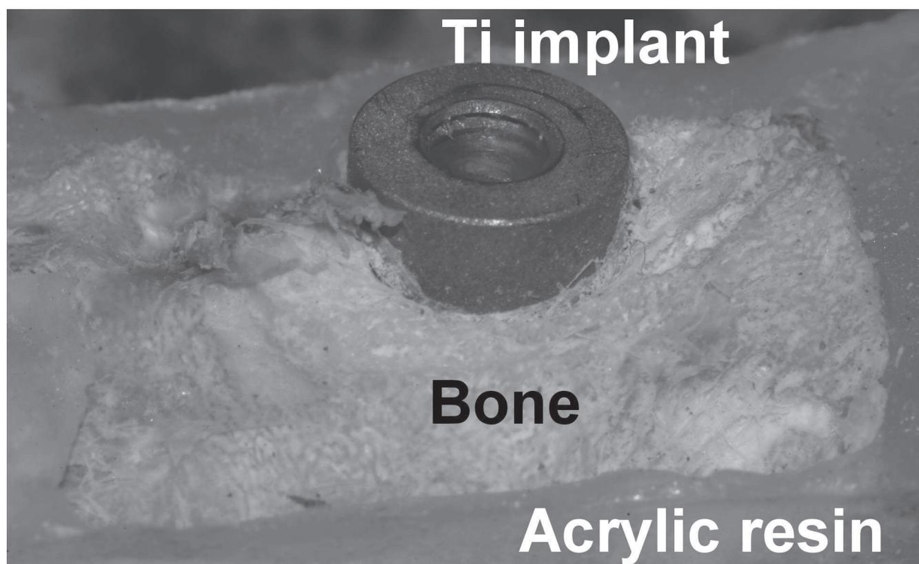
FIGURE 2 - Bone-implant *en bloc* embedded in acrylic resin ready to perform the osseointegration evaluation. The titanium treated surfaces are in contact with the sheep cortical bone
