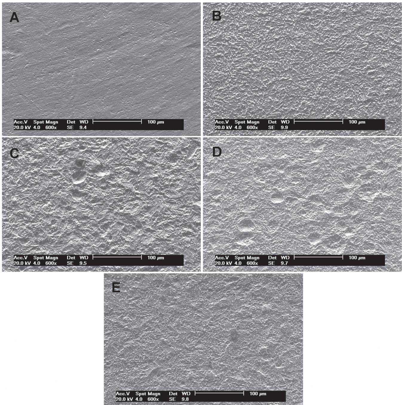
FIGURE 4 - Scanning electron micrographs of Titanium implants after the surface treatments. In (A) Control Group; (B) Group B; (C) Group C; (D) Group D; (E) Group E
