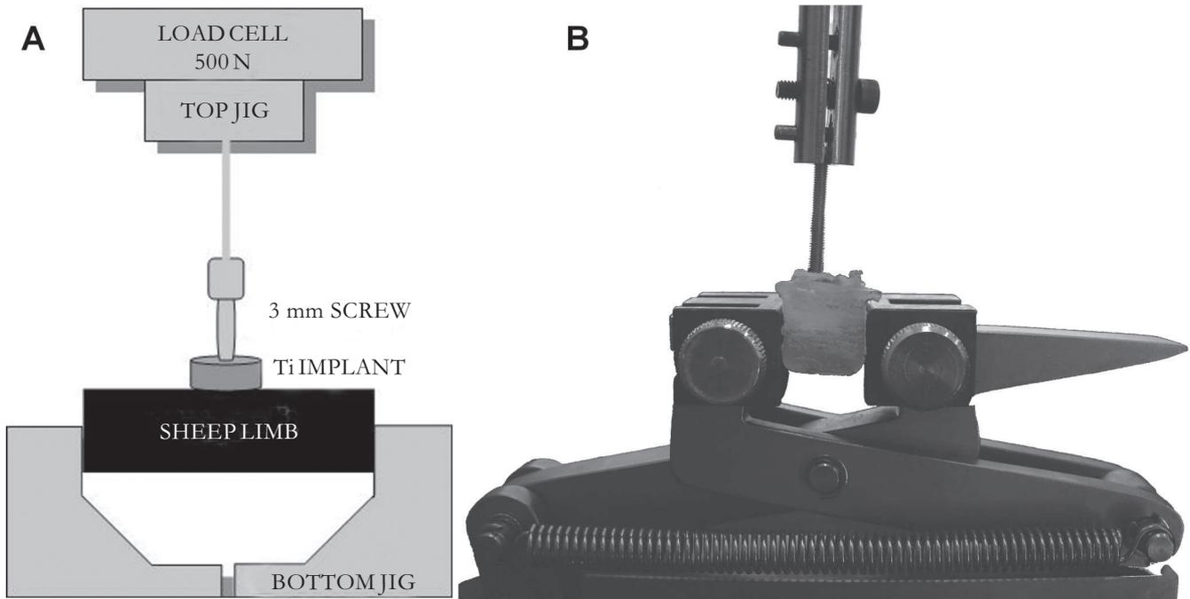
FIGURE 3 - In (A) schematic illustration of the pull out test apparatus. The samples embedded in acrylic resin are fixed in a bottom jig and the top jig is fixed in the ball-head pin located in the through hole of all implants. In (B) the implants are pulled out until the completely rupture of the bone-implant interface
