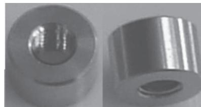
FIGURE 1 - Coin-shaped titanium implants (4 mm in thickness and 6 mm in diameter)
