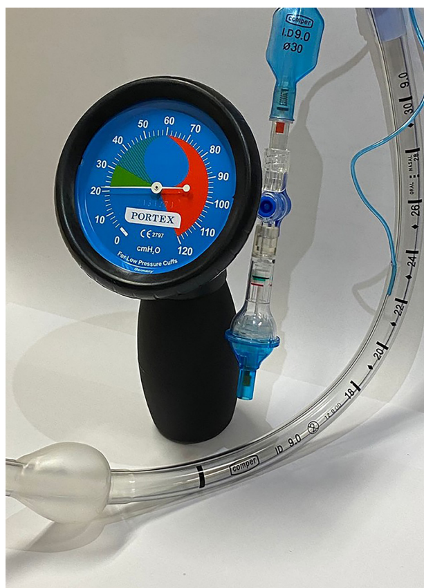
Figure 1 - Bench test of the continuous cuff pressure monitoring device (AccuCuff™ Cuff Pressure Indicator) connected to a conventional handheld cuff pressure manometer via a three-way stopcock.
