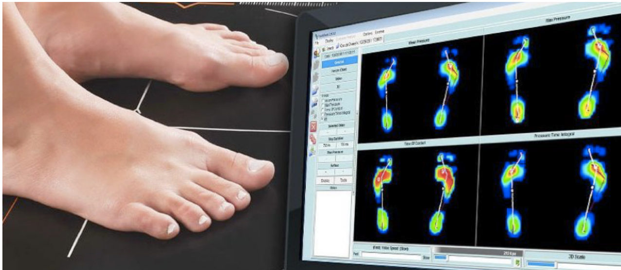
Figure 1 – Records of center of gravity of Footwork® baropodometry platform.
