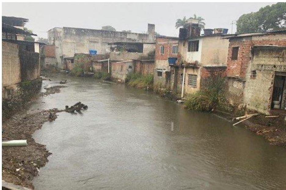
Figure 4 - Jiquiá stream as an example of the urban stream syndrome in Recife, where urbanization has increased flows, causing flood and erosion.
